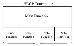
Sub-function on each port implements the HDCP Transmitter State Diagram
