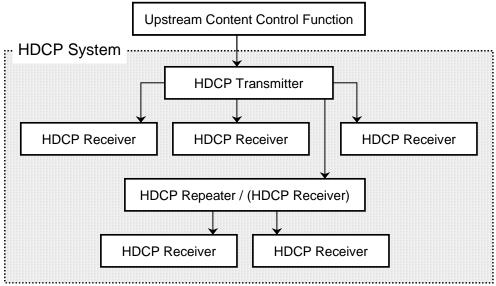
Figure 1.1 illustrates an example connection topology for HDCP Devices.
