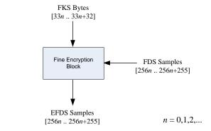
Figure 3.5. Block Division and Sample Ordering for Fine Data Encryption
