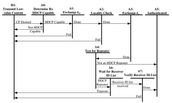
Figure 2.12. HDCP Transmitter Authentication Protocol State Diagram
