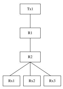
Figure 2.8. DEPTH and DEVICE\_COUNT for HDCP Repeater
