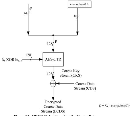
Figure 3.2. HDCP Cipher Structure for Coarse Data
