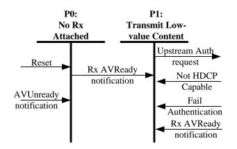
Note: Transition arrows with no connected state (e.g. Reset) indicate transitions that can occur from multiple states
