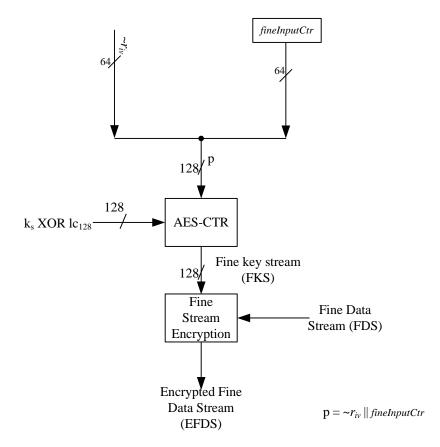
Figure 3.4. HDCP Cipher Structure for Fine Data
