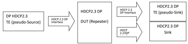
Note: A device that has already passed the DP HDCP2.2 compliance test is used as the Sink device
