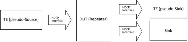
Note: A device that has already passed the compliance test is used as the Sink device
