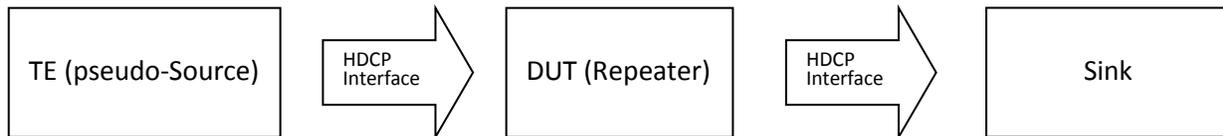
Note: A device that has already passed the compliance test is used as the Sink device
