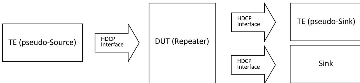
Note: A device that has already passed the compliance test is used as the Sink device
