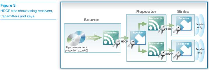
Each HDCP transmitter or receiver includes 40 56-bit secret keys, known as Device Private Keys, as shown in figure 3. These keys, provided by DCP, are unique to the transmitter or receiver, highly confidential and not available to other devices.
