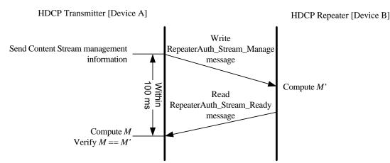
Figure 2.9. Downstream Propagation of Content Stream Management Information
