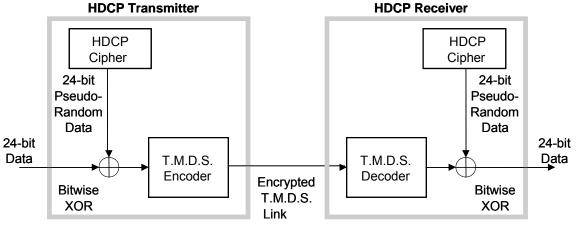
Figure 3.1. HDCP Encryption and Decryption
