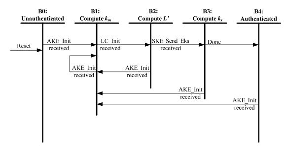
Figure 2.13. HDCP Receiver Authentication Protocol State Diagram
