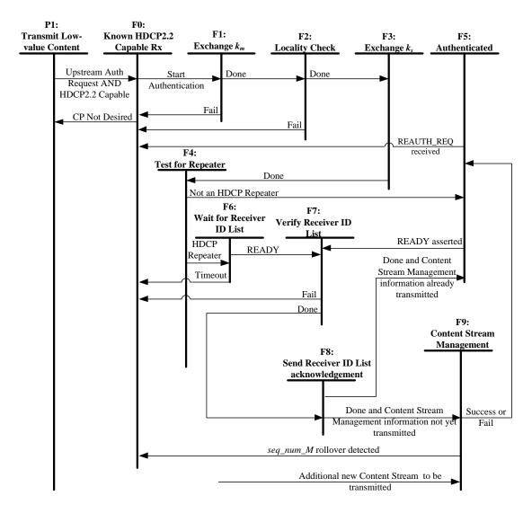
Figure 2.15. HDCP Repeater Downstream Authentication Protocol State Diagram
