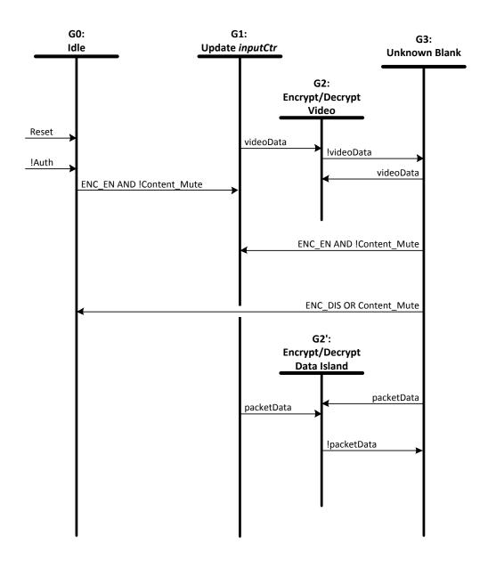
Figure 3.4. Encryption/Decryption State Diagram (EESS)
