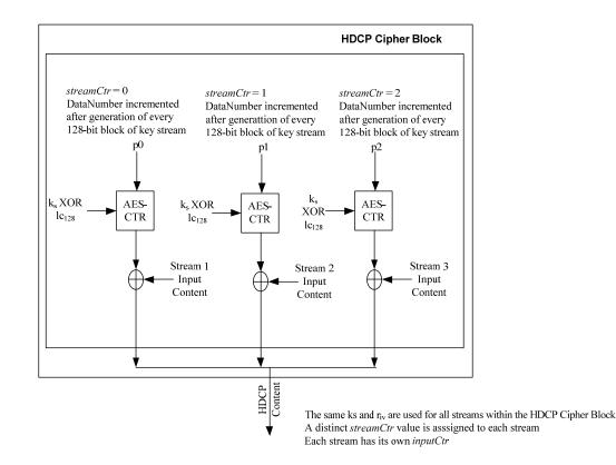
Figure 3.3. HDCP Encryption of Multiple Streams
