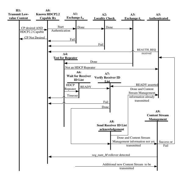
Figure 2.11. HDCP Transmitter Link State Diagram
