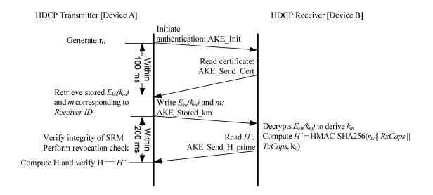
Figure 2.2. Authentication and Key Exchange (With Stored  $k_m$ )
