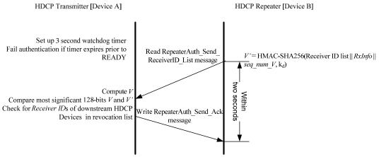
Figure 2.5. Upstream Propagation of Topology Information
