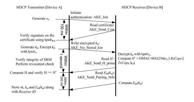
Figure 2.1. Authentication and Key Exchange (Without Stored *k<sub>m</sub>*)
