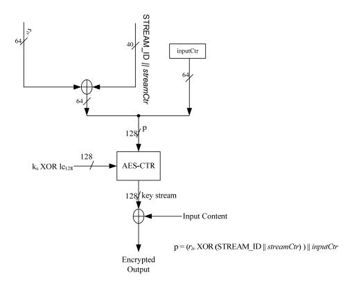
Figure 3.2. HDCP Cipher Structure
