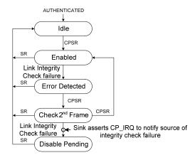
Figure 2-10. HDCP Receiver Link Integrity Check State Machine
