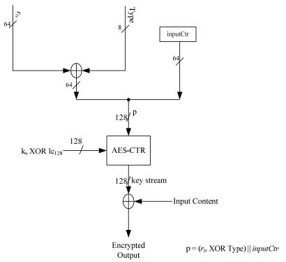
Figure 3-3. HDCP Cipher Structure
