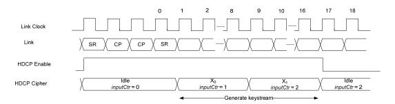
Figure 3-11. 2-Lane HDCP Cipher Operations in SST Mode
