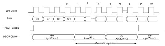
Figure 3-10. 4-Lane HDCP Cipher Operations in SST Mode
