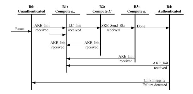
Figure 2.14. HDCP Receiver Authentication Protocol State Diagram
