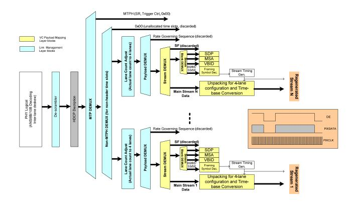
Figure 3-2. HDCP Decryption in the DisplayPort Receiver
