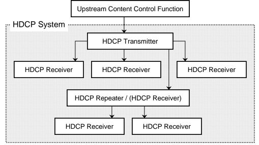
Figure 1.1. Sample Connection Topology of an HDCP System
