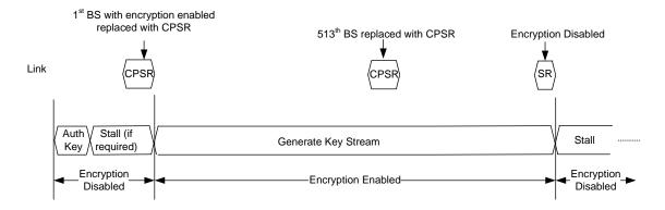
Figure 3-9. Encryption Status Signaling in SST Mode and HDCP Cipher Operations
