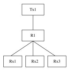
Figure 2.6. DEPTH and DEVICE\_COUNT for HDCP Repeater
