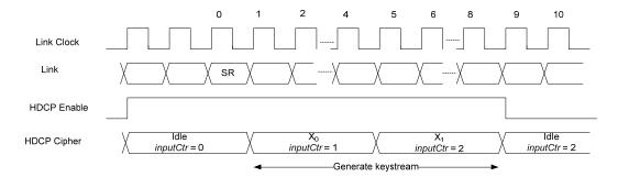
Figure 3-6. 4-Lane HDCP Cipher Operations in MST Mode
