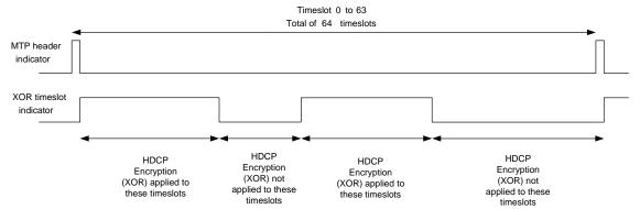
Figure 3-4. HDCP Encryption Applied Based on HDCP\_Encryption\_Control Bits 1:63
