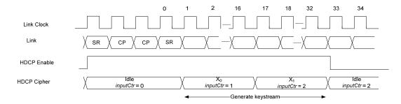
Figure 3-12. 1-Lane HDCP Cipher Operations in SST Mode
