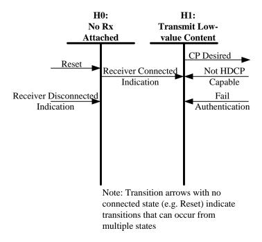
Figure 2.12. HDCP Transmitter Link State Diagram
