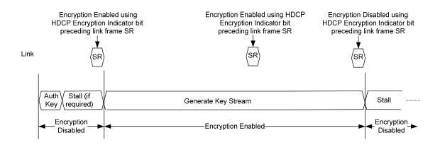
Figure 3-5. Encryption Status Signaling in MST Mode and HDCP Cipher Operations
