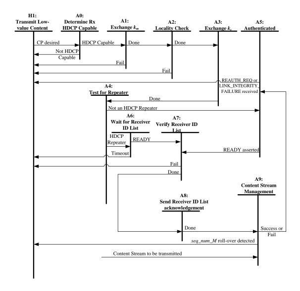
Figure 2.13. HDCP Transmitter Authentication Protocol State Diagram
