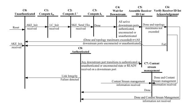
Figure 2.17. HDCP Repeater Upstream Authentication Protocol State Diagram
