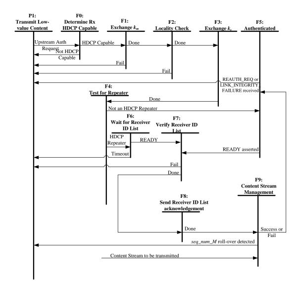
Figure 2.16. HDCP Repeater Downstream Authentication Protocol State Diagram
