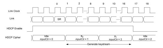
Figure 3-7. 2-Lane HDCP Cipher Operations in MST Mode
