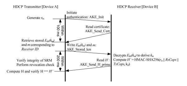
Figure 2.2. Authentication and Key Exchange (With Stored  $k_m$ )
