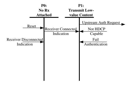
Note: Transition arrows with no connected state (e.g. Reset) indicate transitions that can occur from multiple states
