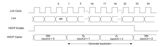
Figure 3-8. 1-Lane HDCP Cipher Operations in MST Mode
