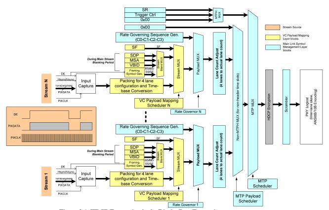
Figure 3-1. HDCP Encryption in the DisplayPort Transmitter
