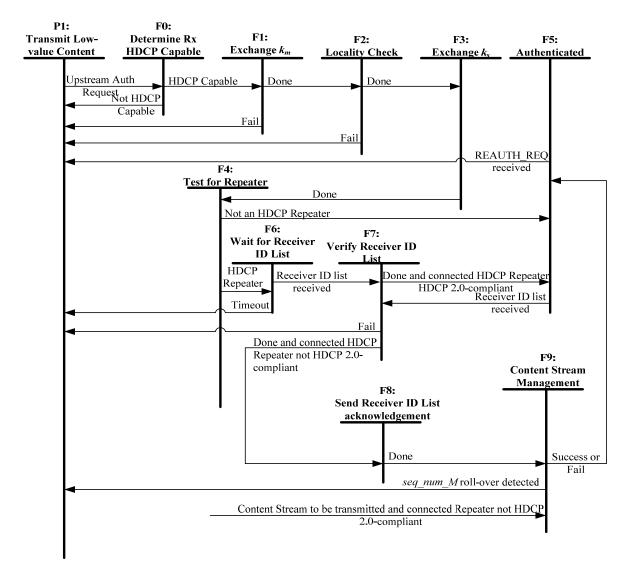
Figure 2.16. HDCP Repeater Downstream Authentication Protocol State Diagram
