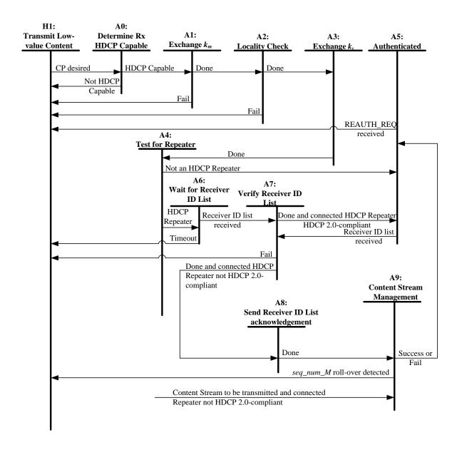
Figure 2.13. HDCP Transmitter Authentication Protocol State Diagram
