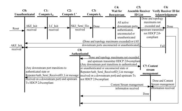
Figure 2.17. HDCP Repeater Upstream Authentication Protocol State Diagram
