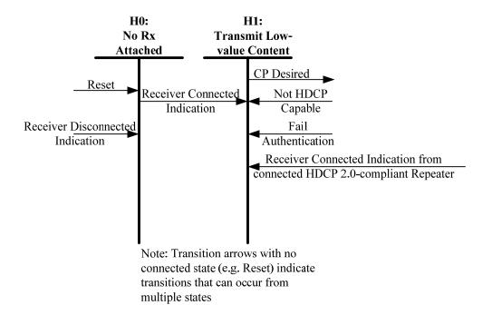
Figure 2.12. HDCP Transmitter Link State Diagram
