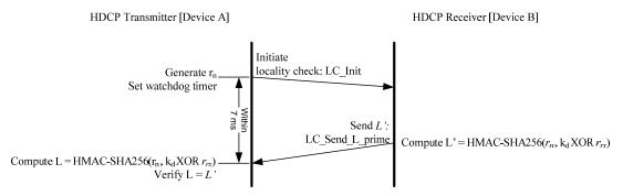
Figure 2.4. Locality Check between HDCP Transmitter and HDCP Receiver
