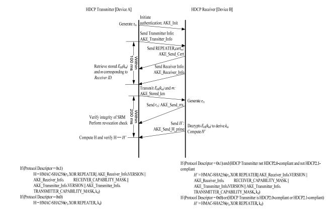
Figure 2.2. Authentication and Key Exchange (With Stored  $k_m$ )
