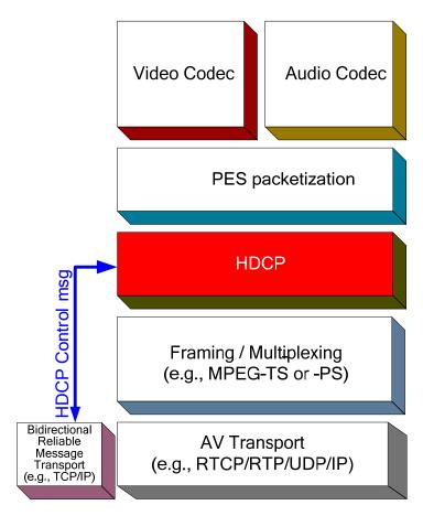
Figure 3.1. Transport Protocol w. HDCP Block Diagram (Informative)
