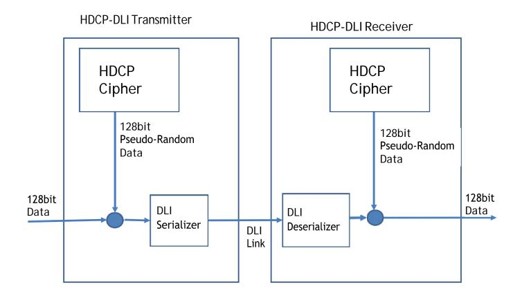
Figure 1: HDCP-DLI Encryption Diagram
