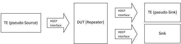
Note: A device that has already passed the compliance test is used as the Sink device
